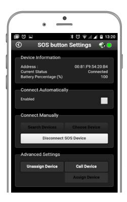
Once connected, you can "Call" the SOS Button device (for example to locate it) and of course you can "Unassign" it.
